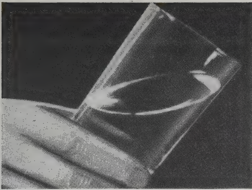
When we cut a cylinder by a plane, we get an ellipse.
